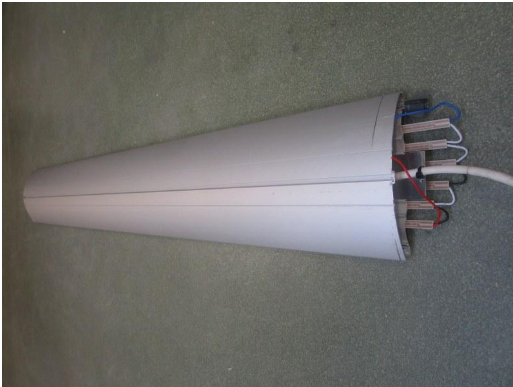
Photo 7 Visual inspection. IP6X. No dust observed inside enclosure.
