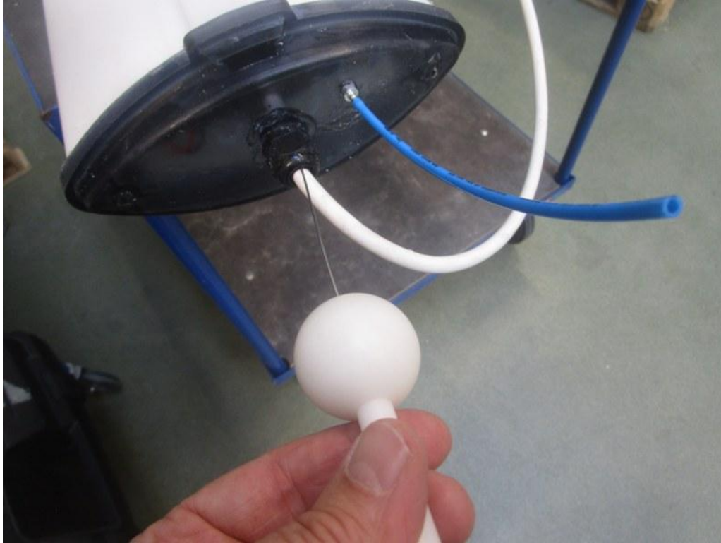
Photo 10 Enclosure protection IP5X. Ø1.0 mm probe could not enter the enclosure and clearance was kept.
