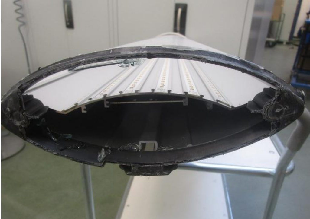
Photo 4 Visual inspection. IP6X. No dust observed inside enclosure.
