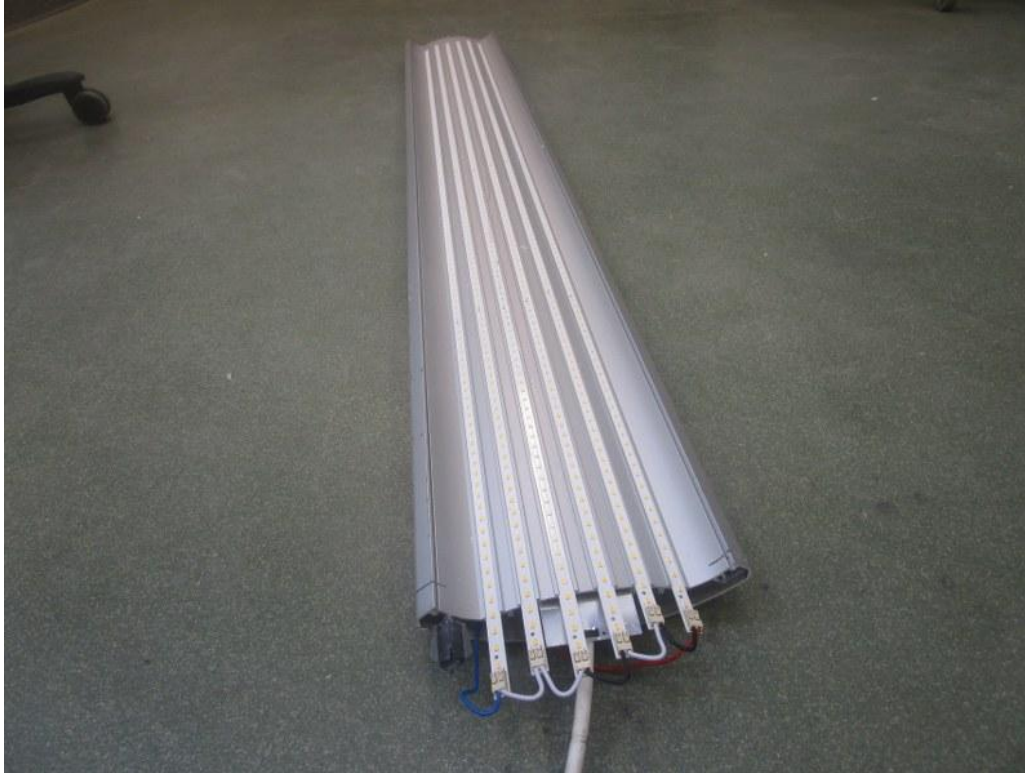
Photo 6 Visual inspection. IP6X. No dust observed inside enclosure.
