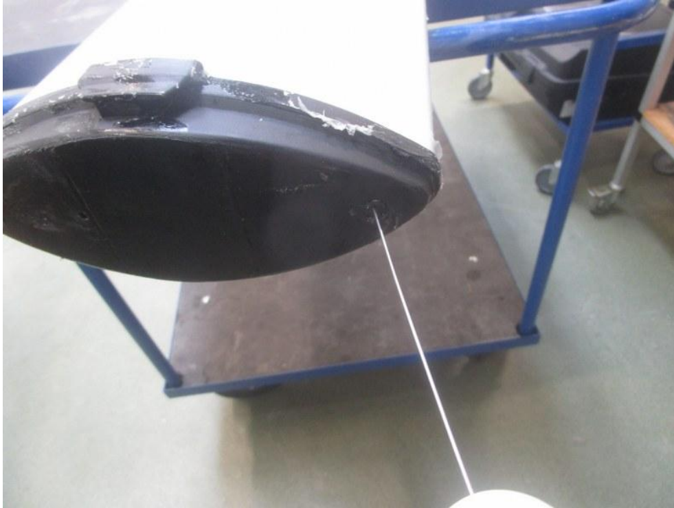
Photo 12 Enclosure protection IP5X. Ø1.0 mm probe could not enter the enclosure and clearance was kept.
